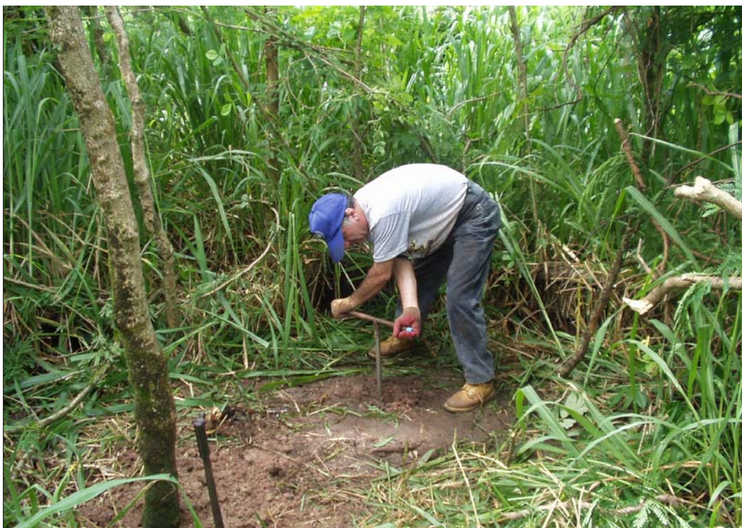
Plate 6: Coring lysimeter insertion holes with soil auger downgradient of Ordot Landfill
