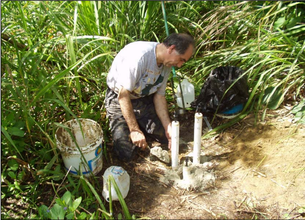
Plate 7: Seating the lysimeter in position with soil slurry and packing with fine sand
