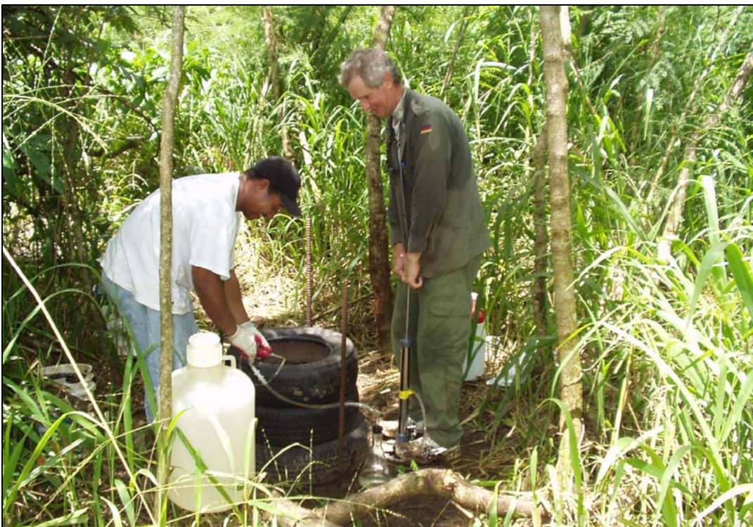
Plate 8: Removing soil pore water sample from lysimeter with vacuum pump.
