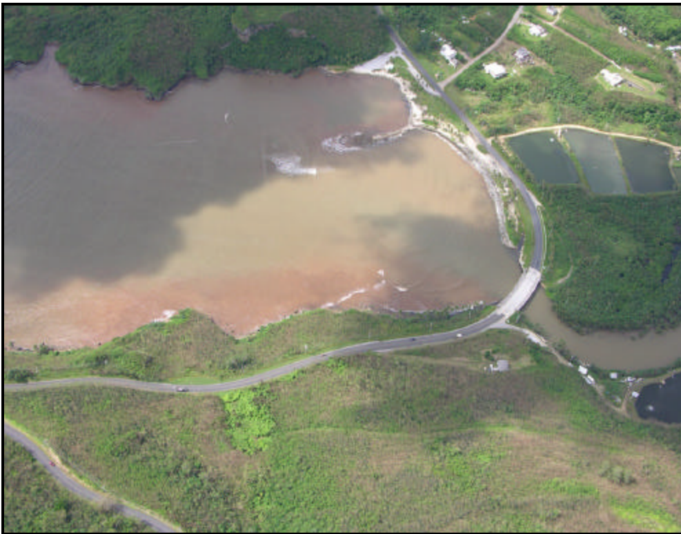
Figure 4. Talofofu Bay after heavy rainfall event. The bay is choked by sediment washed down from the Talofofu and Ugum River systems.
