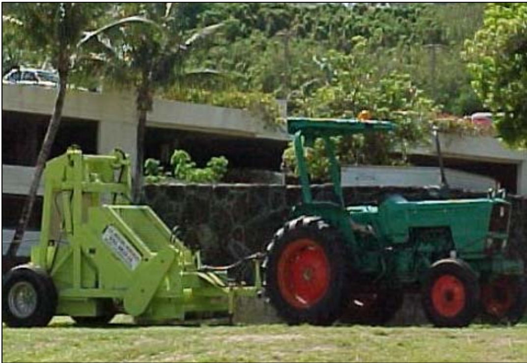
Plate 4: Tractor drawn mechanical sand-rake used daily for beach cleaning in Tumon Bay
