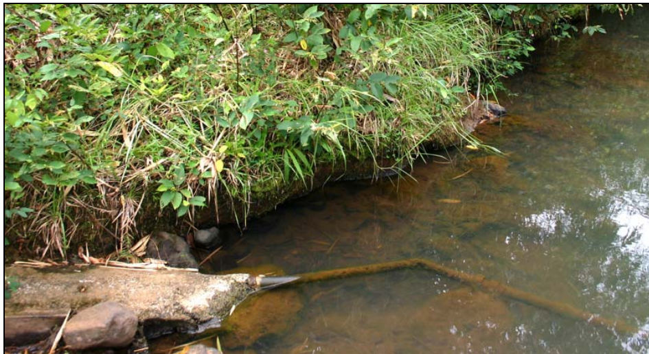
Figure 27: Photo of the submerged pipe connected to the Ugum River gage and sediment sampler station (USGS Station 16854500)
