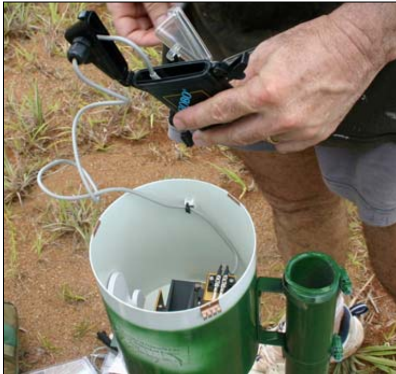
Figure 29: Close-up view of the electronic recorder called HOBO attached to the Rain gage # 1.
