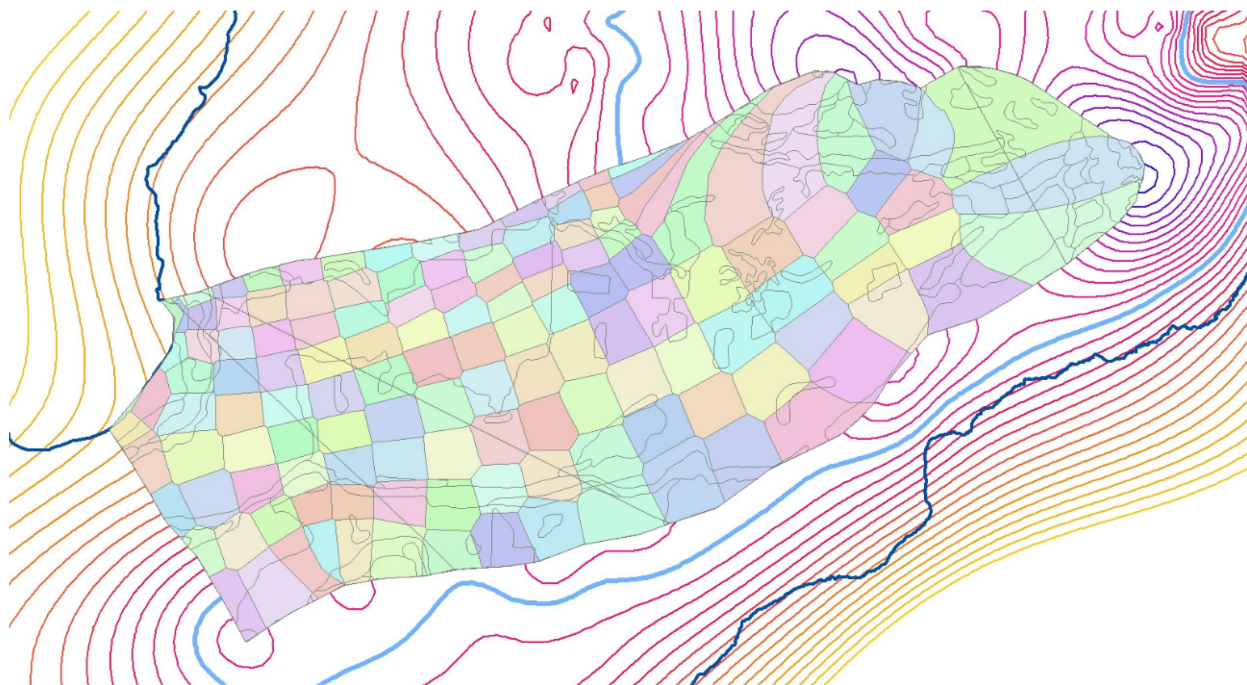
Figure 50. Final union of rain, pan evaporation, soils, and node-sheds. This completes the node-shed model surface construction.
