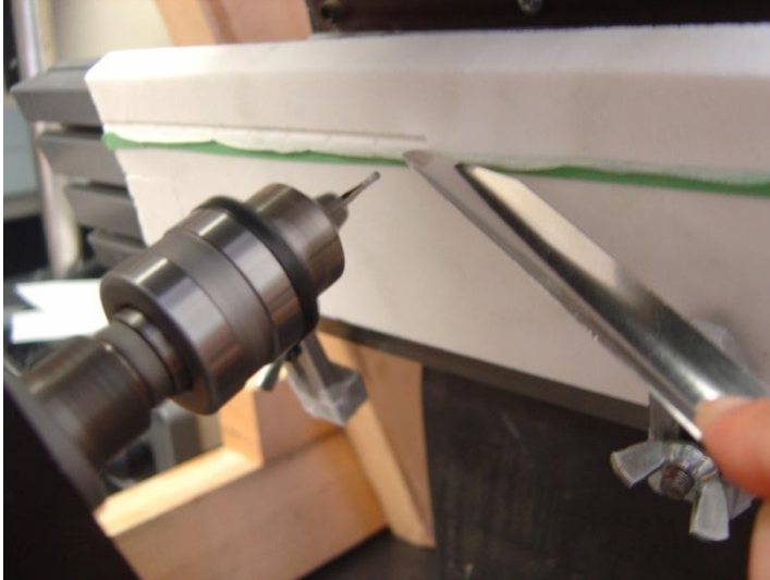
Figure 23. The procedure to prepare 616 samples by computer controlled Micro-Mill.
