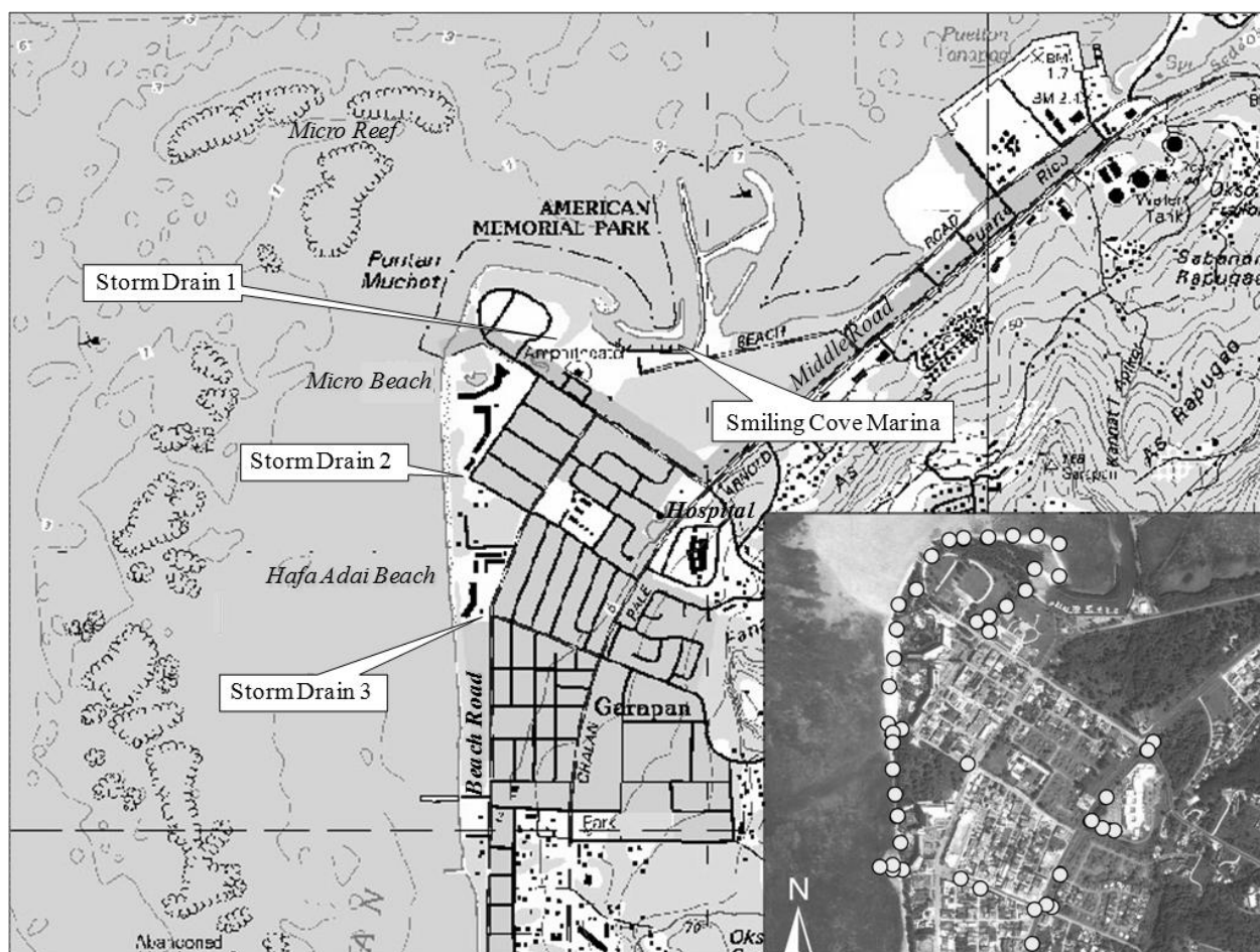
Fig.2 USGS topographic map of Garapan village, Saipan, showing storm drain locations and known potential sources of mercury pollution relative to Hafa Adai Beach
