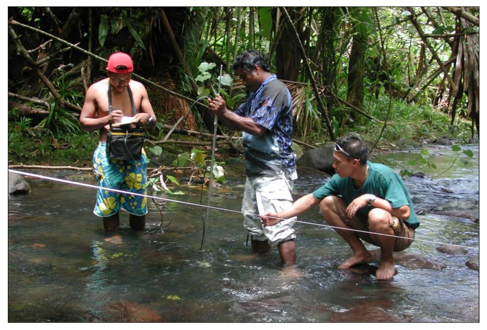
WERI hydrology students in the Environmental Science MS Program learn how to calculate stream flow measurements in the Lonfit River, Guam
