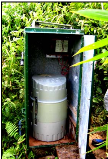
Ugum Stream Sediment Sampler
