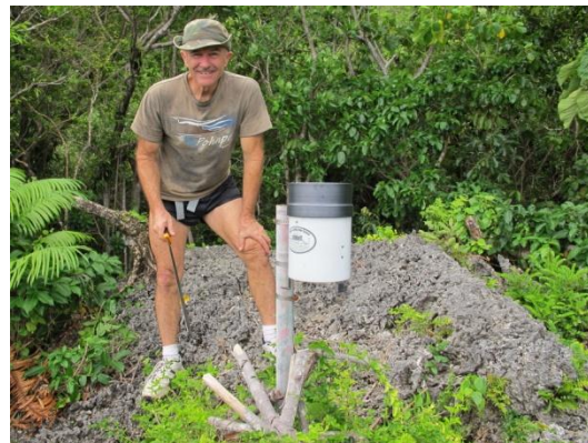
Dr. Mark Lander with installed rain gauge in northern Guam.
